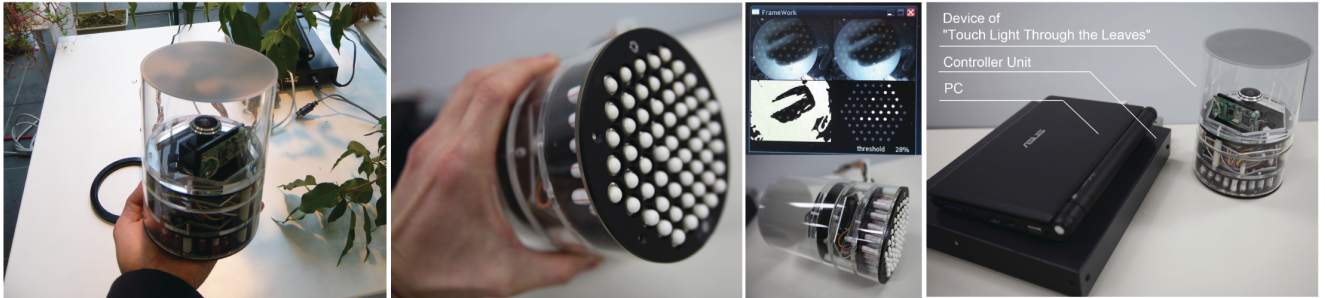
Figure 1: Left: Picture of "Touch Light Through the Leaves, Center Left: Tactile display with vibration units, Upper Center Right: Detection result of light and shadow by the camera and determination of vibration units, Lower Center Right: Side view of the tactile display, Left: System overview
